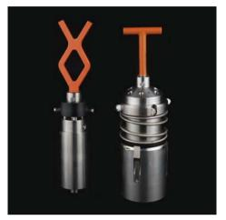
The ClampOn Ultrasonic Intelligent Sensor processes all data in the sensor itself (patented principle), thus enabling the instrument to discriminate between sand-generated and flow-generated noise. This is of importance to the user since changes in flow rates and the gas/oil ratio will not affect the performance of the system.
